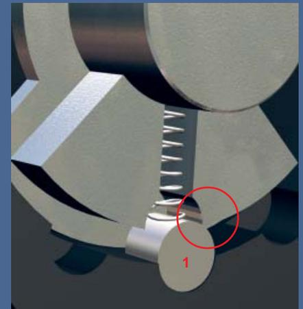
It's in this position that the security bolts (1) effectively prevent the turning of the window handle from outside. The window handle locks and foils the attempted break-in.
